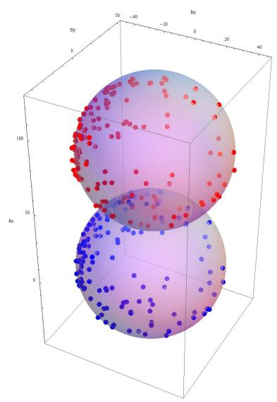
Figure 3-1: Uncalibrated (Red) and Calibrated (Blue) Measurements from a Simple Hard Iron Environment
