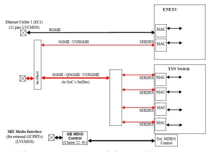
ENETC and switch management, SoC sees 4 different network interfaces (instances of our Ethernet controller) 2 of which are connected to ports of the switch using back-to-back MAC connections
