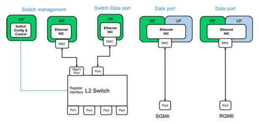
The TSN Switch IP is a 6-port TSN-capable Ethernet switch. 4 of the 6 ports operate at
