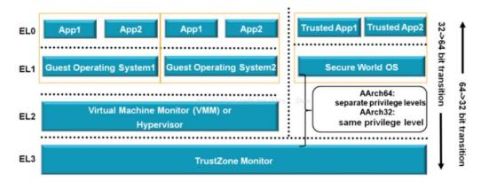
OP-TEE is based on ARM TrustZone to provide isolation of the TEE from the rich OS. Please refer to the following Trustzone architecture in software perspective.
