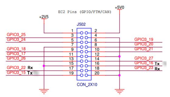
Figure 68. Hardware diagram for the FlexCan demo
