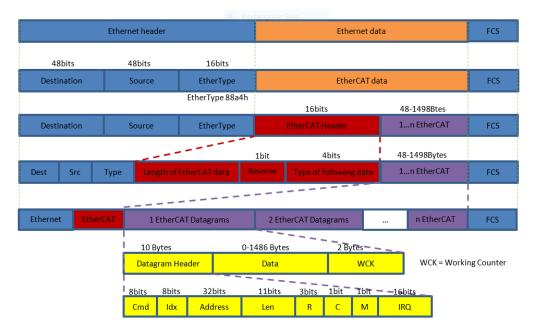
Figure 58. EtherCAT frame structure
