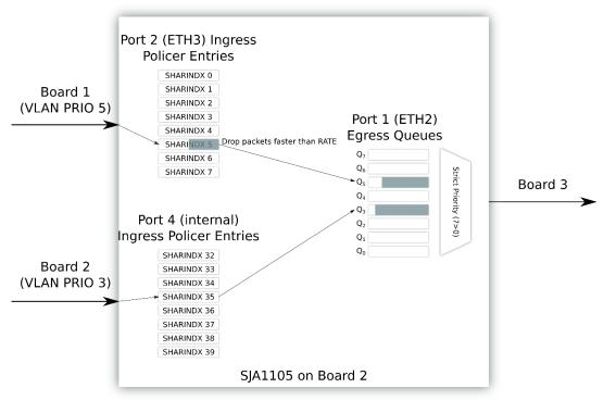
Figure 40. Queuing diagram for policing configuration
