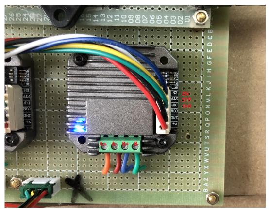
Figure 61. Stepper motor driver
