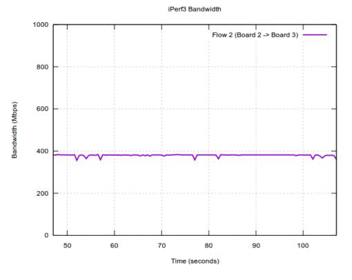
Figure 47. Scheduling configuration: Flow 2 run by its own
