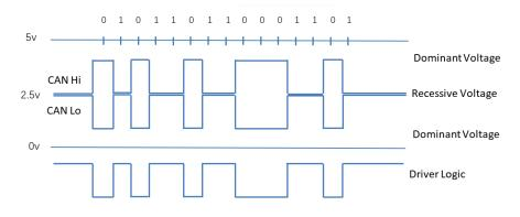
Figure 64. High speed CAN signaling
