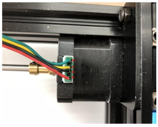
Figure 62. Stepper motor
