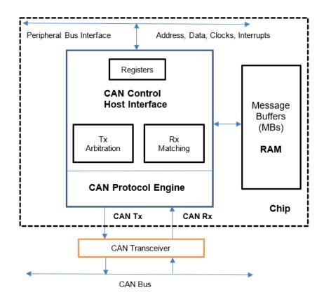
Figure 63. FlexCAN block diagram
