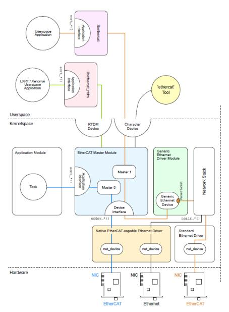
Figure 57. IGH EtherCAT master architecture
