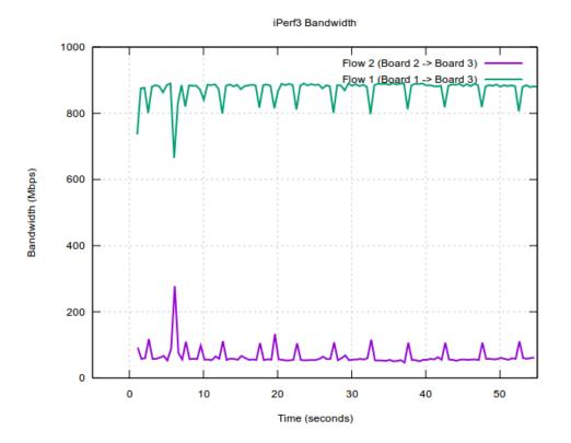
Figure 39. Prioritizing configuration: both flows run at the same time
