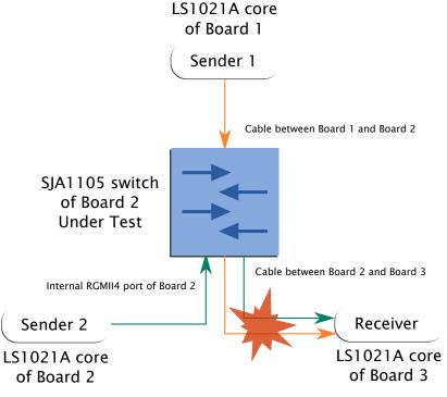
Figure 30. Simplified traffic flows for the rate limiting use case
