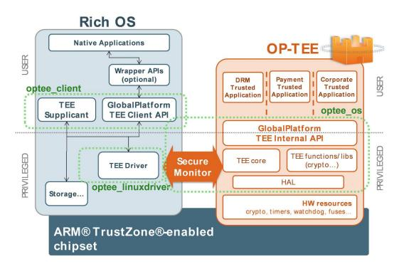
Figure 8. Architecture of OP-TEE on an ARM TrustZone enabled SoC
