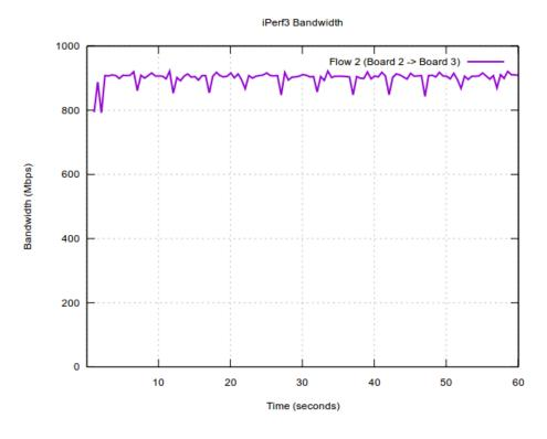
Figure 38. Prioritizing configuration: Flow 2 run by its own
