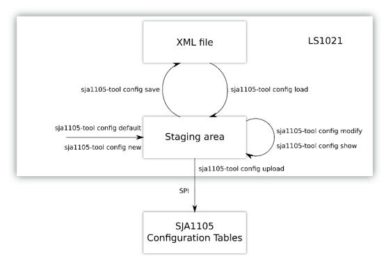
The physical SPI registers of the SJA1105 switch are write-only. Therefore, a copy of these registers is kept in the staging area, which is effectively a file in the LS1021A OpenIL filesystem. The staging area keeps a binary image of the configuration to be uploaded over SPI using sjall05-tool config upload, and can also be read back by the user with sjall05-tool config show.
