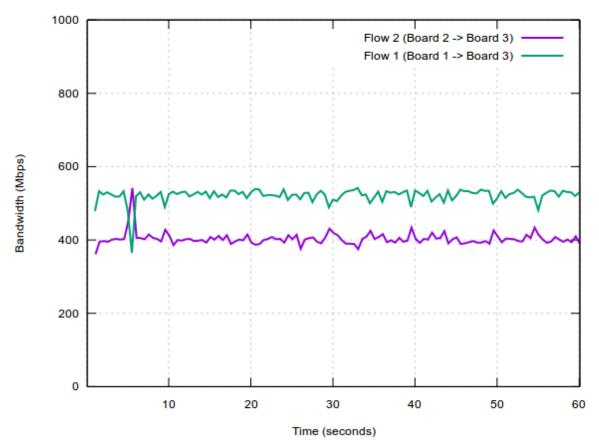
Figure 43. Policing configuration: both flows running at the same time
