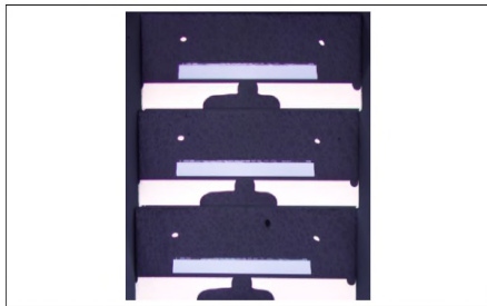
Figure 3. Photo of the cross-section showed internal package structure.
