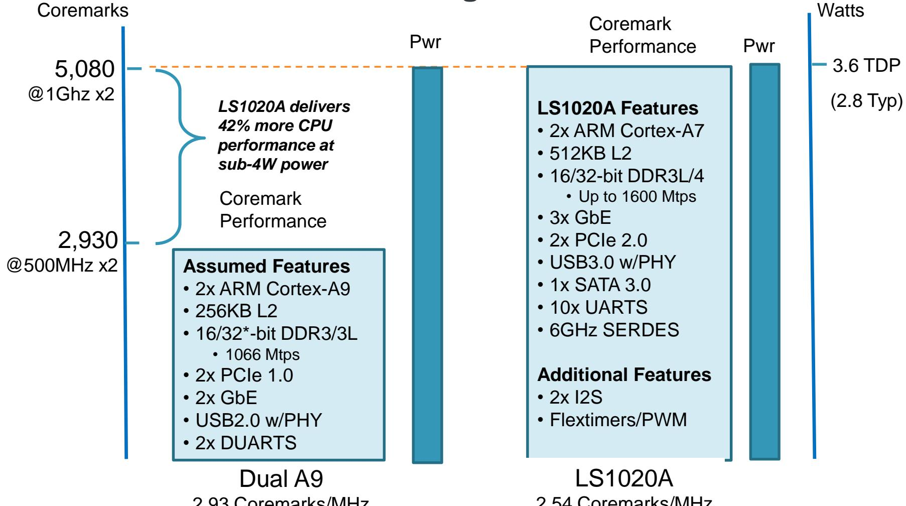
At same power, 2x ARM Cortex-A7 based QorIQ LS1020 processor achieves 42% higher performance compared to 2x ARM Cortex-A9 based SoC
