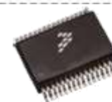
EK SUFFIX (PB-FREE) 98ASA10556D 32-PIN SOICW-EP
