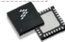
ES SUFFIX (PB-FREE) 98ASA00656D 32-PIN QFN (WF-TYPE)
