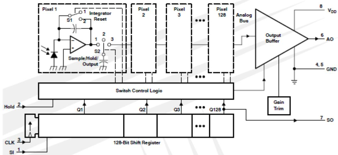
The sensor consists of 128 photodiodes arranged in a linear array. Light energy impinging on a photodiode generates photocurrent, which is integrated by the active integration circuitry associated with that pixel. During the integration period, a sampling capacitor connects to the output of the integrator through an analog switch. The amount of charge accumulated at each pixel is directly proportional to the light intensity and the integration time."
