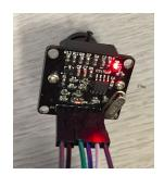
analog signal(green), digital signal or D1 signal (blue), field sync signal (white), and line sync signal (purple).
