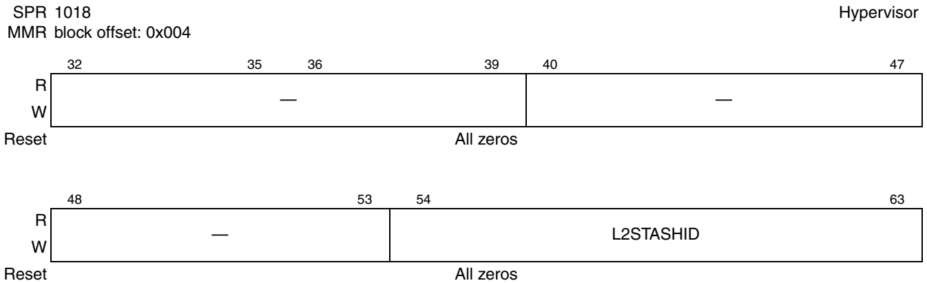
Figure 3-52. L2 Cache Control and Status Register 1 (L2CSR1)
