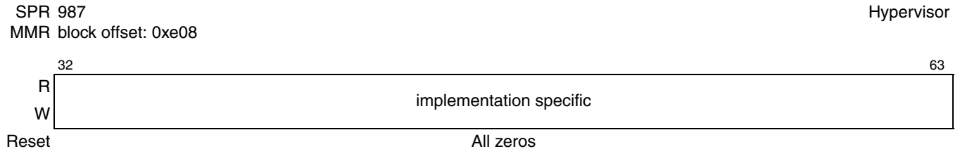
Figure 3-63. L2 Cache Error Injection Control Register (L2ERRINJCTL)
