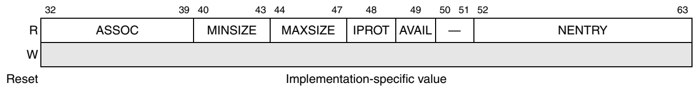
Figure 3-70. TLB Configuration Register n (TLB0CFG)
