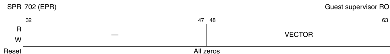
Figure 3-38. External Proxy Register (EPR)
