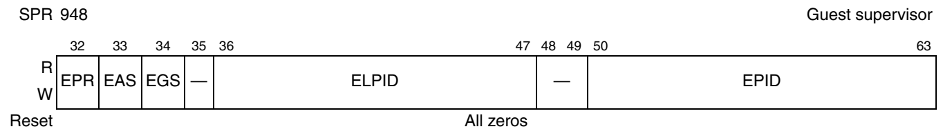
Figure 3-81. External PID Store Context (EPSC) Format
