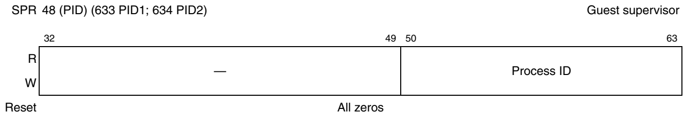
Figure 3-67. Process ID Registers (PID, PID1, PID2)
