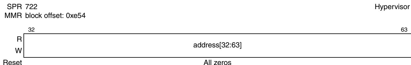
Figure 3-58. L2 Cache Error Address Capture Register (L2ERRADDR)
