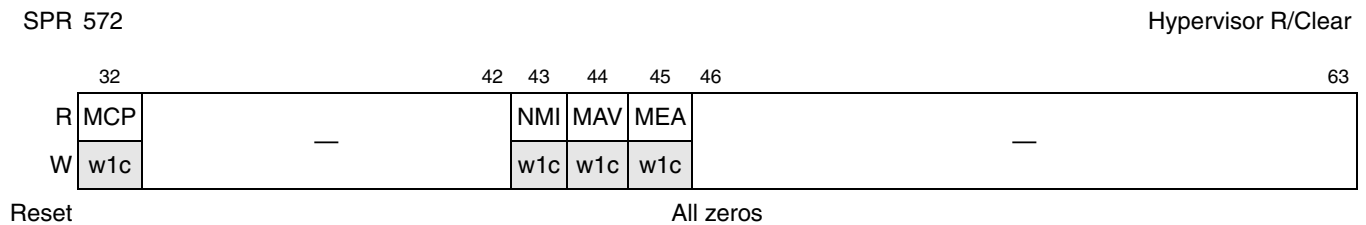
Figure 3-36. Machine Check Syndrome Register 1 (MCSR)
