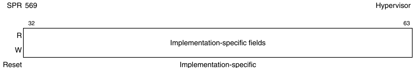
Figure 3-89. Debug External Control Register 0 (DBECR0)
