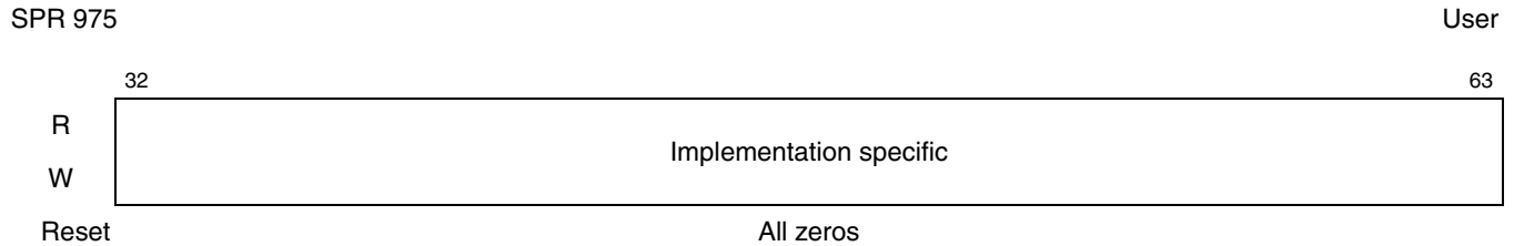
Figure 3-97. Debug Event Register (DEVENT)
