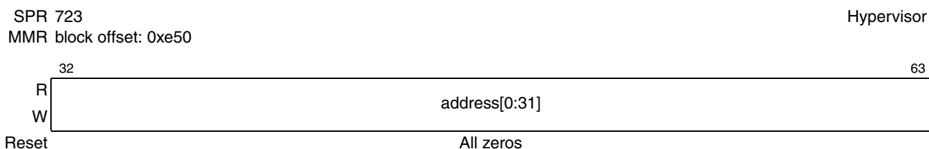
Figure 3-59. L2 Cache Error Extended Address Capture Register (L2ERREADDR)
