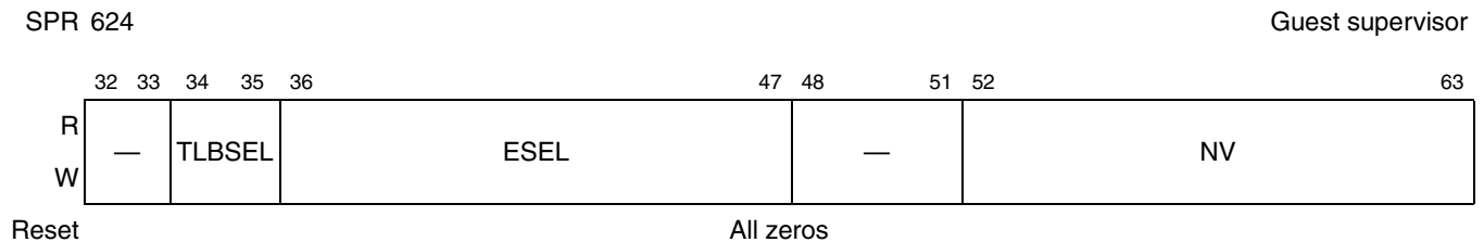
Figure 3-71. MAS Register 0 (MAS0)
