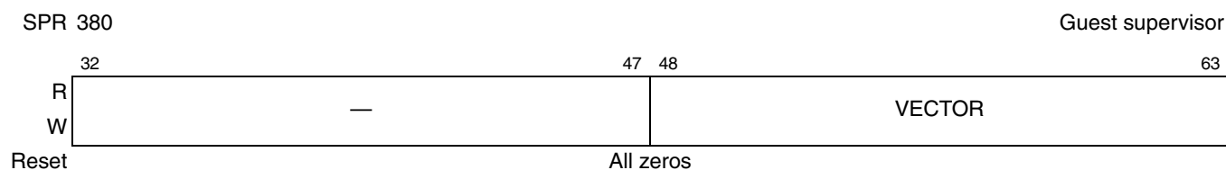
Figure 3-39. Guest External Proxy Register (GEPR)
