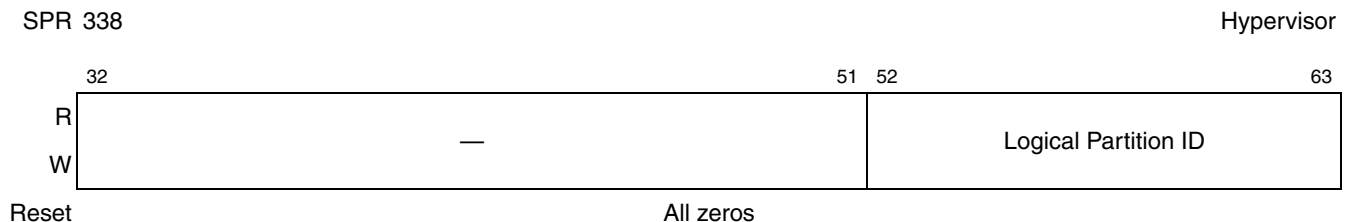
Figure 3-66. Logical Partition ID Register (LPIDR)
