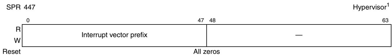
Figure 3-29. Guest Interrupt Vector Prefix Register (GIVPR) Format
