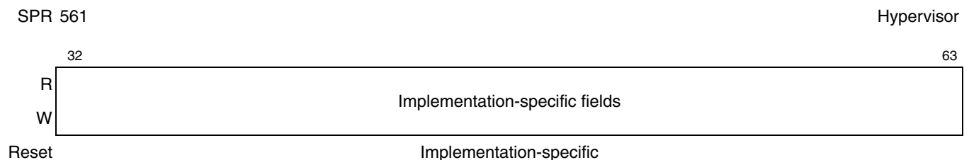
Figure 3-85. Debug Control Register 3 (DBCR3)
