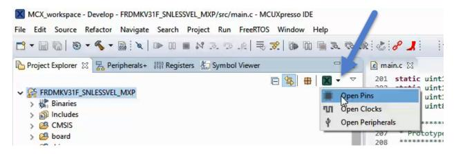
Make the changes needed to the pin assignments. When you have completed the changes to the pin assignments make sure to update the project code by clicking on the *Update Project Code* button.
