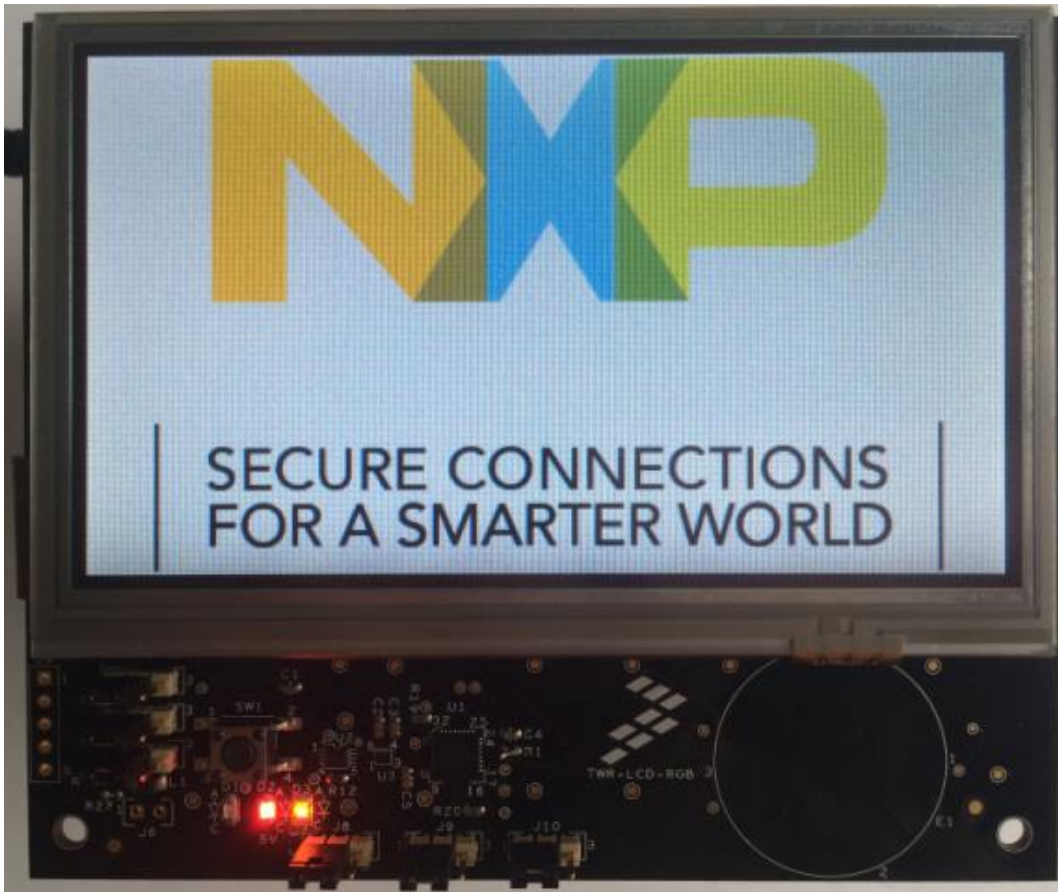
Figure 1. TWR-LCD-RGB driven by FlexIO
