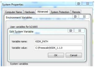
IMPORTANT NOTE: If you installed more than one KSDK or MQX for KSDK versions you must be sure that KSDK\_PATH variable is pointing to the correct installation.
