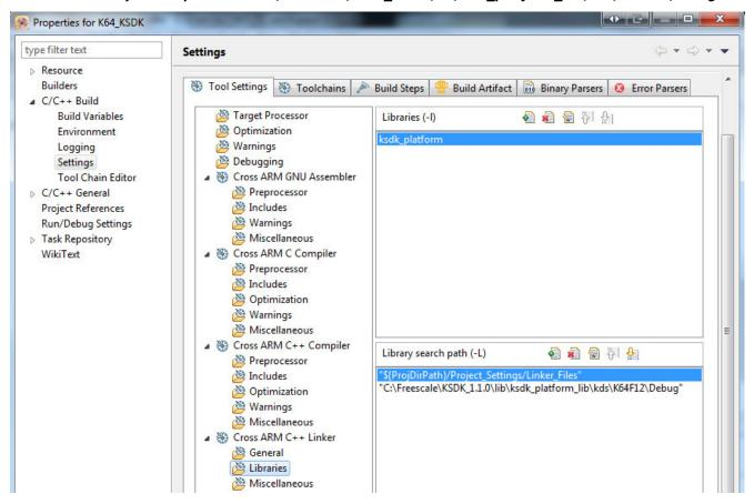
**NOTE:** At this point '*libksdk\_platform*'must be built, please refer to step 1.5 - It is necessary to build KSDK Platform Driver Library (libksdk\_platform.a)' on this document.
