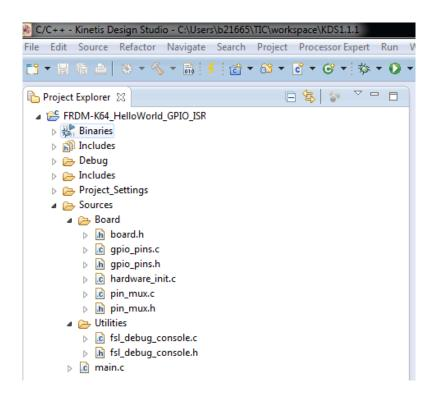
3.7 Go to menu Project > Properties C/C++ Build > Settings > Cross ARM C Compiler > Includes and add to 'Include paths (-I)' the path "../Sources/Board". DO NOT COPY-PASTE this line because quotes cause problems when copy-pasting.
