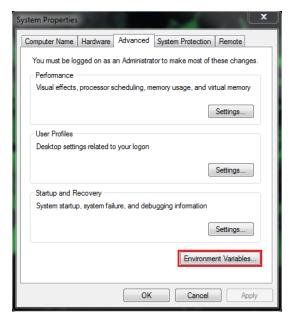
1.1 If the variable does not exists click 'New' button under 'System variables' to create 'KSDK\_PATH' variable. The path must be where KSDK is installed. The default path is 'C:\Freescale\KSDK\_1.1.0'. If the variable exists but it does not point to your KSDK installation folder click 'Edit' button to correct it.
