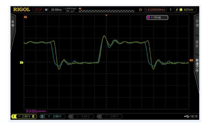
The code can demonstrate the fractional duty cycle(nano-edge placement), it runs on TWR-KV46F150M with OSBDM mode plus primary Elev board.
