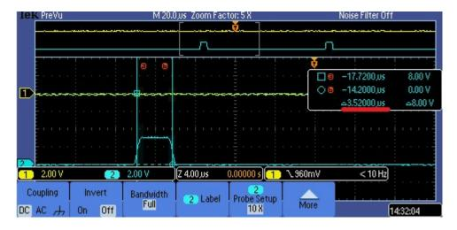
Figure 6: freertos example timing after optimization
