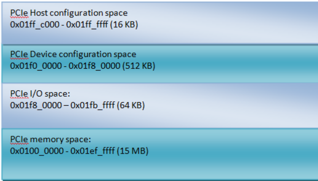
Figure 42-2. Memory Layout (i.MX 6Quad/6DualLite/6Solo)
