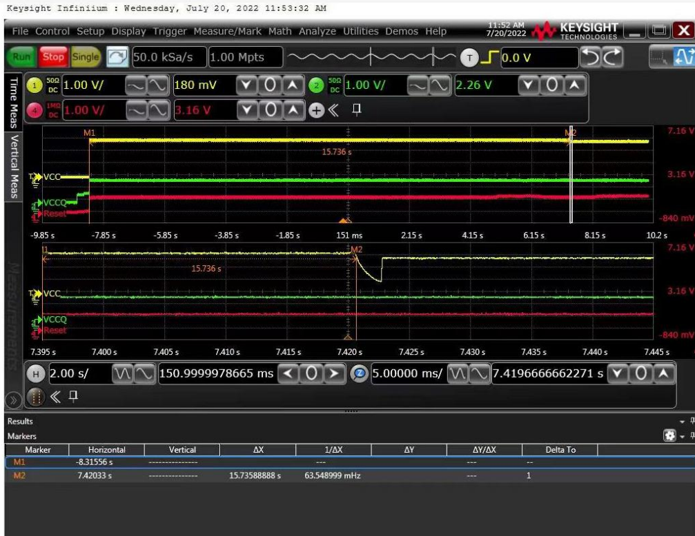
Figure#4: Platform#1—Anormal Vcc drop was found after power up 15s
