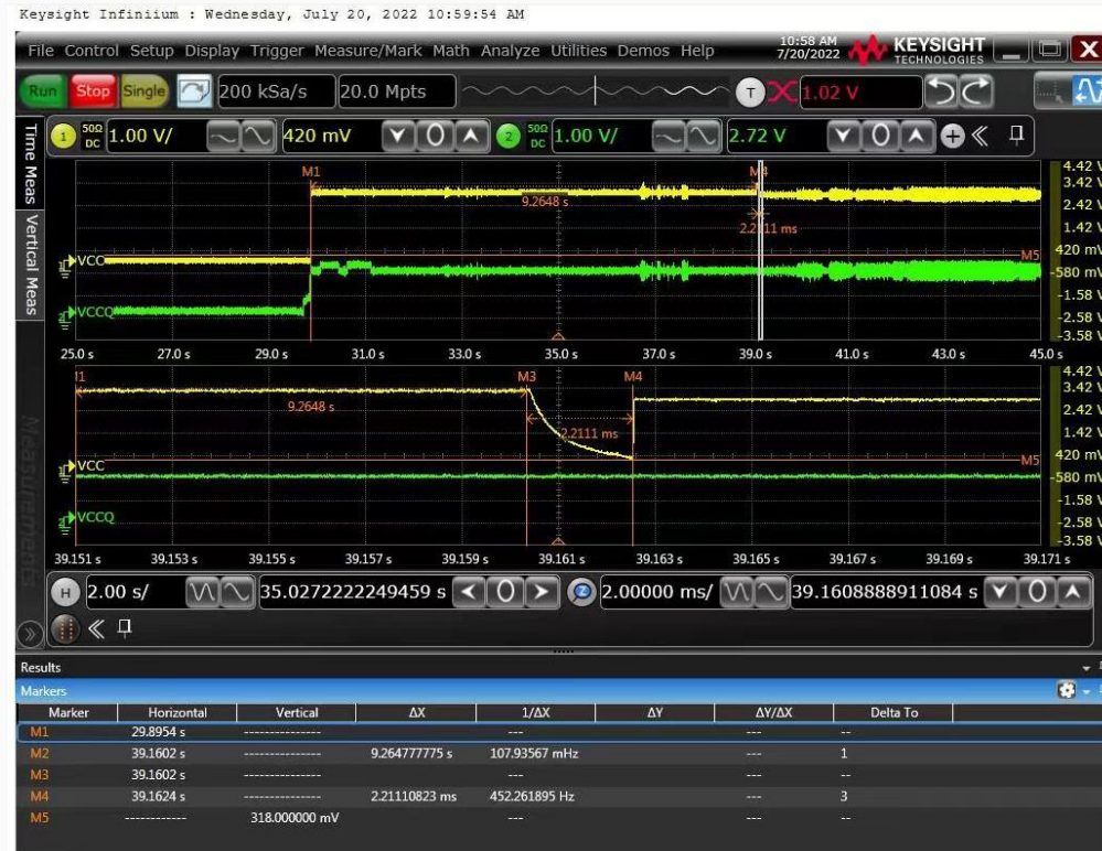
Figure#5: Platform#2—Anormal Vcc drop was found after power up after 9s
