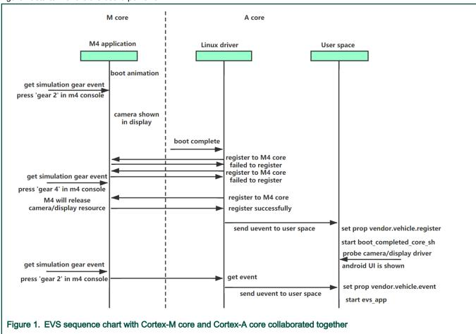
Rear view camera (RVC) is only supported in Android cars. The following is the registration process of the vehicle client.
