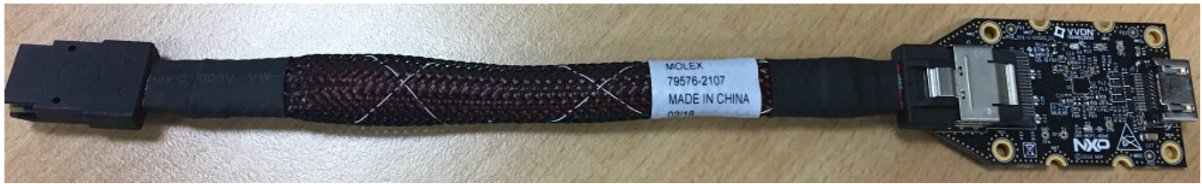
Figure 15. i.MX mini SAS cable with DSI-to-HDMI adapter
