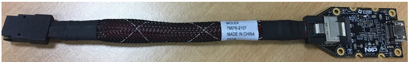
Figure 10. i.MX mini SAS cable with DSI-to-HDMI adapter
