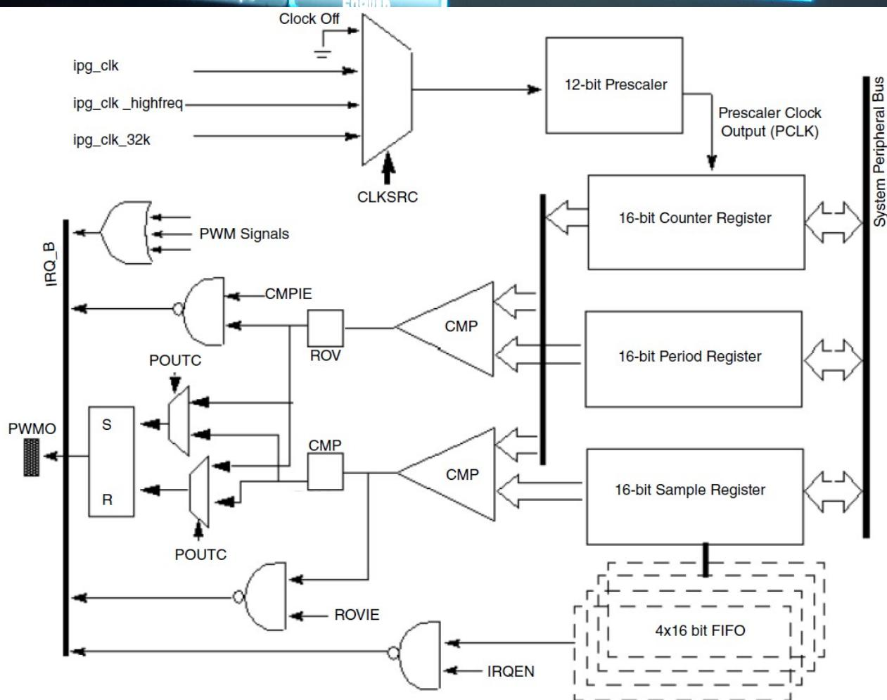
This is a Scalable PWM Modulator based on the infamous NXP PWM Peripheral present on an Toradex Colibri imx7 module, M4 core suitable for driving current through LED(s) or controlling brightness/contrast on a display and even perhaps motor control with some adjustments.
