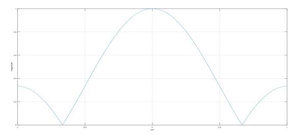
From the AFR diagram, we can see that three-point average system is FIR low pass filter (Also known as Nonrecursive Discrete-Time Filter.)
