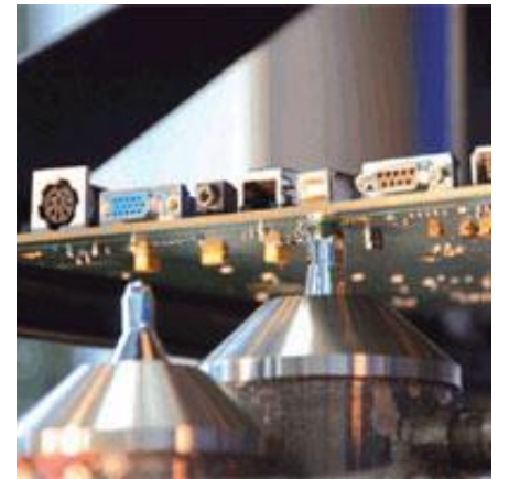
Selective Soldering Process
