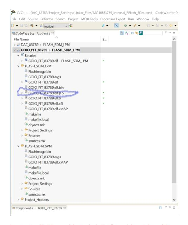
Note that the \*.elf.p.S file can only be downloaded by blhost tools instead of the \*.elf.S. Restriction: ROM bootloader puts its global variable into RAM from x:0x0000 and has no protection for them. If we use ".S" or ".x.S" files, it may corrupt ROM bootloader's variables. So let's use ".p.S" file with ROM.
