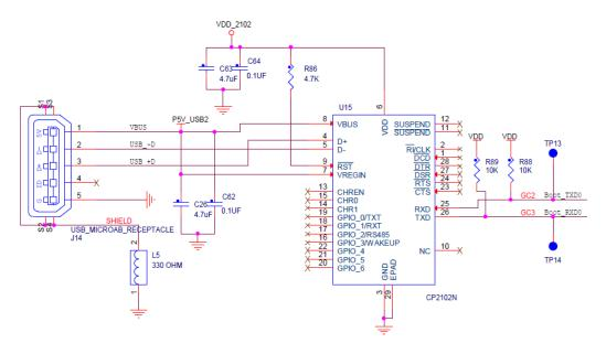
After the J14 USB is connected, the USB port is enumerated as virtual serial port as the following Fig in Computer Device Manager.
