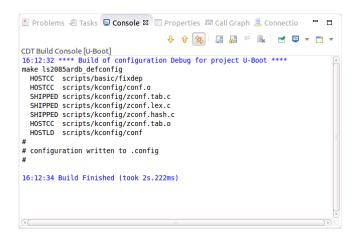
To build U-Boot, go to **Project > Build Project** from the menu bar. Below message will be displayed when build is complete in **Console** view.
