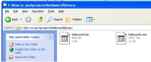
3. Simply "drag and drop" the helloworld.bin or the helloworld.srec file into the FreedmKL25Z drive and the KL25Z128 will be automatically programmed with the pre-compiled binary.
