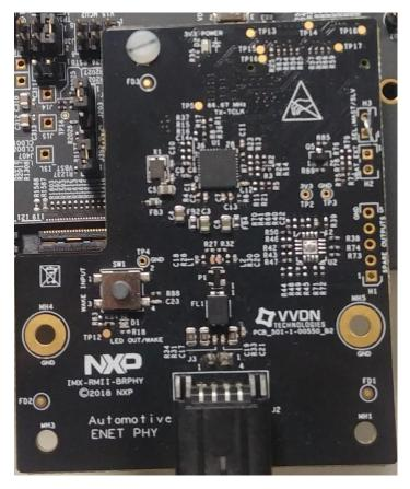
100BASE-T1 MEDIACONVERTER NXP from Technical Engineering GmbH – Setup as master with both switches to On position.
