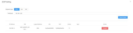
Then user can click connect button, the tool will send **active router** DOIP message firstly, if receive a success response, the TCP socket about this address is stable.
