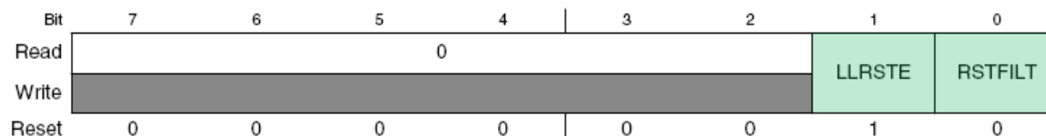
Figure 18. LLWU_RST—New register Rev. 2.x
