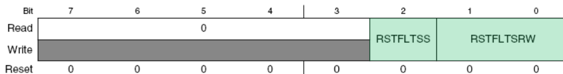
Figure 11. Reset Pin Filter Control Register (RCM_RPFC)—New in Rev. 2.x
