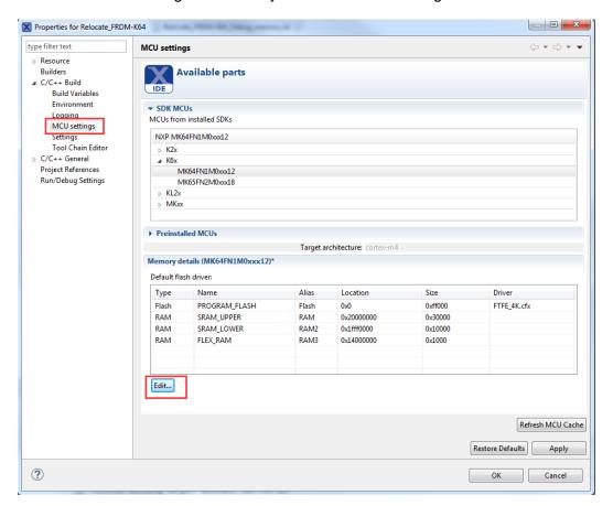
Click the "Edit..." button to add delete or change memory size. By default, the use of "Manage linker script" is enabled for projects. This mechanism allows the MCUXpresso IDE to automatically create a script for each build configuration. So after finish configuring, build, it will create three linker script files for the memory details configuration .
