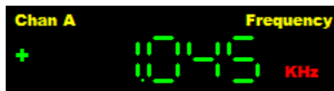
PWM output signal with the factory trim value as Internal Reference clock.
