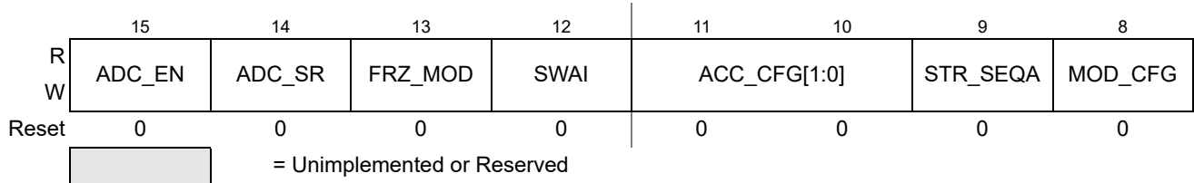
Figure 9-4. ADC Control Register 0 (ADCCTL_0)
