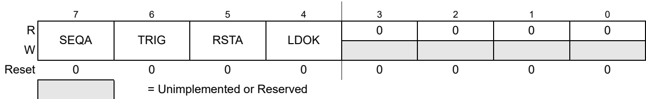
Figure 9-9. ADC Conversion Flow Control Register (ADCFLWCTL)
