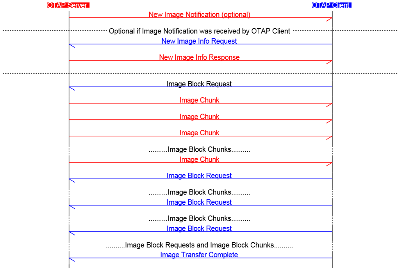
Figure 13. Typical BLE OTAP Image Transfer Scenario Message Sequence Chart
