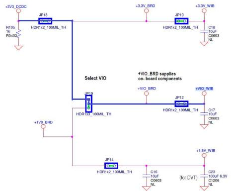
VIO\_WIB determines IW416 IO level, Because we need 3.3V UART, so here, JP13 needs a jumper, JP19 pin1 & pin2 needs a jumper, JP12 needs a jumper, VIO\_WIB will be 3.3V See bold blue line in above schematic, please!
