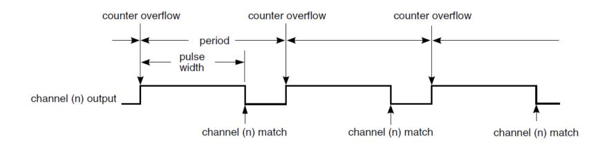
[ELSnB:ELSnA = 1:0] High-true pulses (clear Output on match, set Output on reload)
