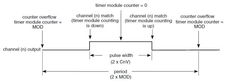
[ELSnB:ELSnA = 1:0] High-true pulses (clear Output on match-up, set Output on match-down)
