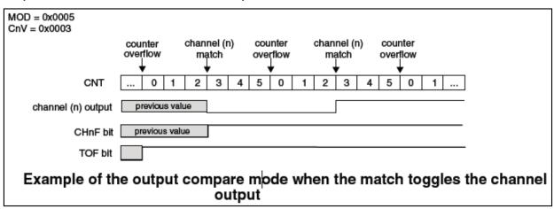
In output compare mode, the TPM can generate timed pulses with programmable position, polarity, duration, and frequency. When the counter matches the value in the CnV register of an output compare channel, the channel (n) output can be set, cleared, or toggled.
