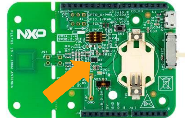
NTAG 5 boost eval board OM2NTA5332 , Arduino shield connectors 10x10mm(!) antenna
