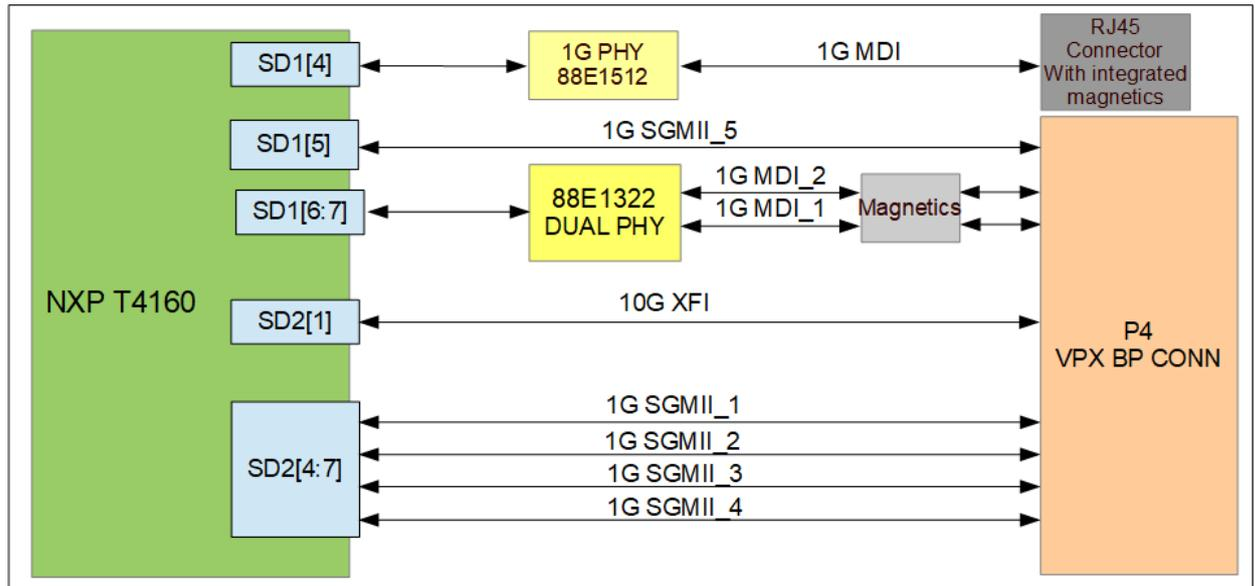
The VPX board has a total of Eight 1G ethernet interface, out of which five 1G SGMII signals are connected to the VPX backplane connector P4 and the other three SGMII is connected through a PHY. Out of the three PHY SGMII signals, two are connected to a dual phy(Marvell 88E1322)and the MDI signals connected to the backplane connector P4 through magnetics, and one SGMII is connected to a single phy(Marvell 88E1512) and it's MDI signals connected to front panel RJ45 connector on board.
