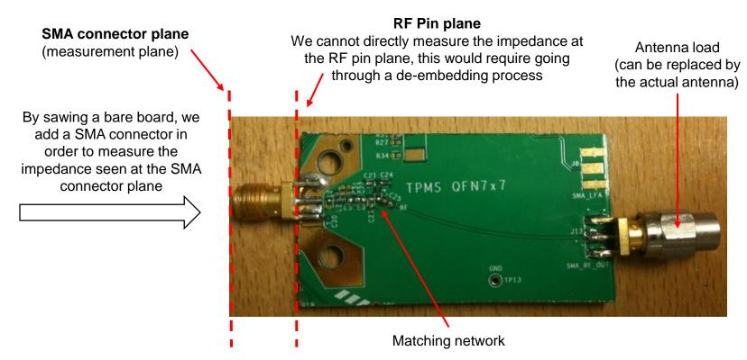
The impedance at the **SMA connector plane** giving the optimized output power was measured and is:
