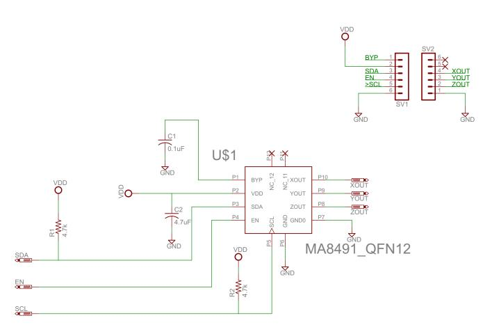
A capacitor must be connected to the Bypass pin (pin 1) to assist the internal voltage regulator. It is recommended to use a 0.1 µF capacitor. The capacitor should be placed as near as possible to the Bypass pin.
