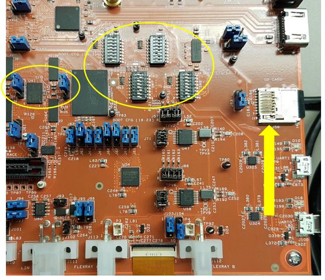
Note: Not all configurations of switches are supported by Linux BSP. Please refer to Linux BSP User Manual for validated modes.
