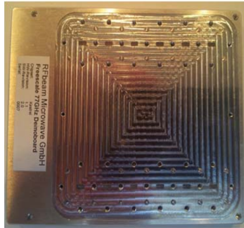
Figure 5. Mechanical Waveguide Transition Adapter (Antenna Side)
