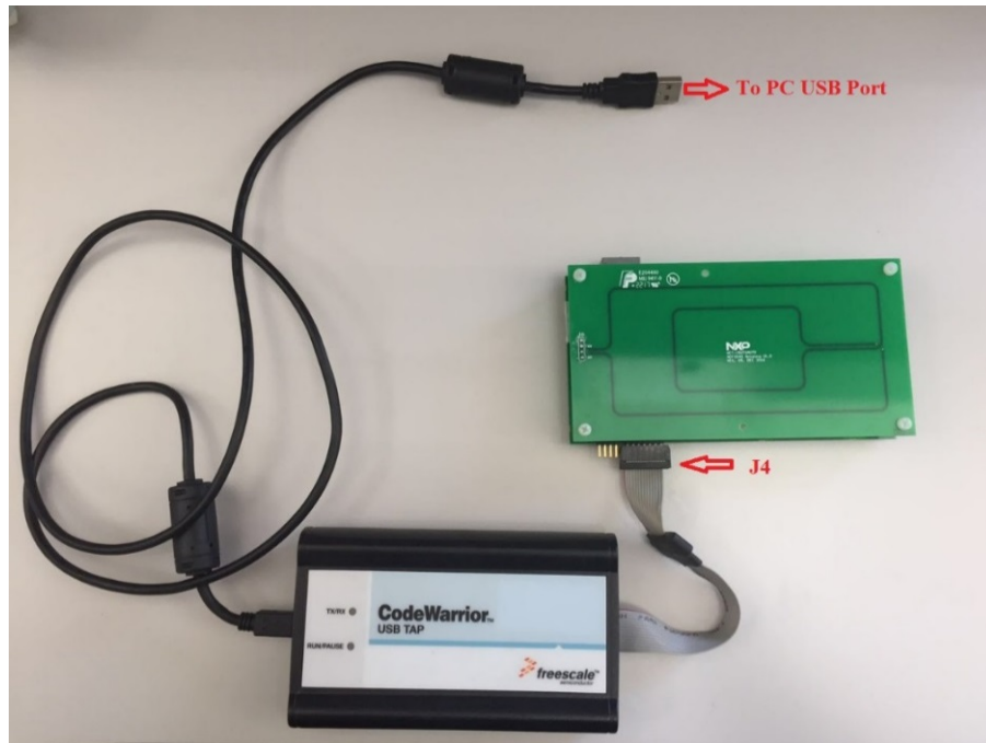
Figure 30. Connecting the debug cable to the board
