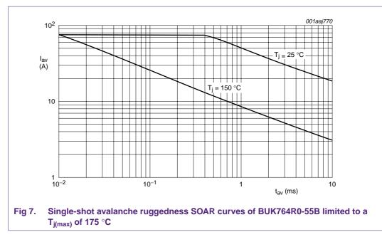
Figure 7 shows the SOAR curves of a device single-shot avalanche capability. The 25 °C junction temperature curve shows the maximum allowable  $I_{AS}$  for a given  $t_{AV}$  at an initial  $T_j$  of 25 °C. This maximum  $I_{AV}$  will give rise to a maximum junction temperature,  $T_{jrise(max)}$  of 150 °C resulting in a  $T_{j(max)}$  of 175 °C.
