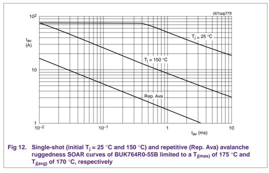
The two conditions which must be satisfied for safe operation of a power MOSFET under repetitive avalanching mode are as follows:
