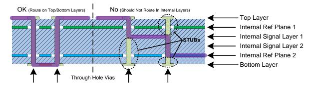
Solid internal reference ground planes should be designed immediately underneath or above the high-speed transmission lines. The distance between the two differential traces should be kept equal as long as possible. Try to avoid vias in the transmission lines themselves. If it is required to use a via, make sure the trace branches to the vias are symmetrical, and oval-shape anti-pads should be used on all internal planes for transitional vias as show in Figure 7 below.
