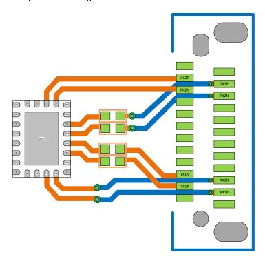
In the next layout example below, even the RX1 signal pairs are routed with minimum number of vias, but the vias are not placed at the optimum position. This layout causes TX1 signal traces to have 2 extra vias that will impact the signal integrity. This should be avoided.
