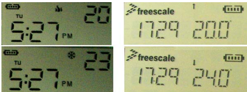
Figure 4-4. Heating and cooling set points
