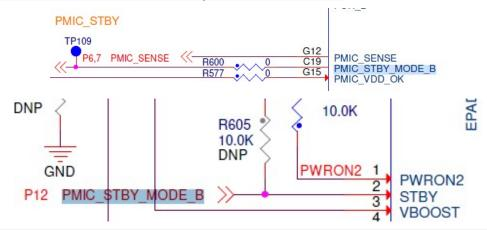
S32G notifies PMIC to enter or exit Standby by pulling PMIC\_STBY\_MODE\_B pin, so you can check whether S32G has entered Standby state by measuring the level change of TP109. This pin level switch is a hardware behavior.
