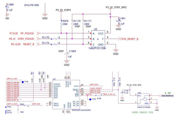
Therefore, after STBY exits, PMIC is powered on, and then pulls STBY\_PGOOD to notify the peripherals to exit STBY. At this time, the external QSPI NOR will be reset, so that when STBY exits, when the M core is doing full boot, QSPI NOR will reset to the initialization state, ensuring bootup successfully.
