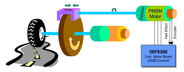
Figure 2-7. EMB Unit detail
