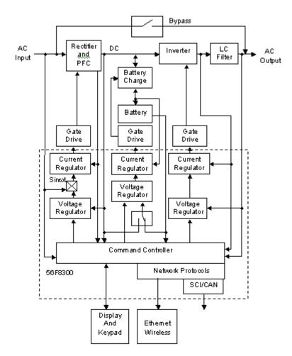
Figure 2-2. UPS Functional Block Diagram
