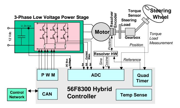
Figure 2-4. Digital Electric Power-Assisted Steering
