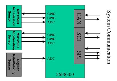
Figure 2-9. Intelligent Inertial Sensor with Three Variables 56F8300 Controller Family, Rev. 1
