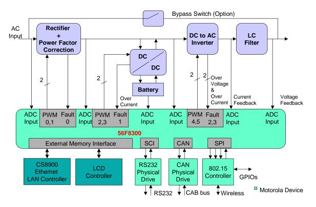
Figure 2-1. Network-enabled UPS Hardware Diagram
