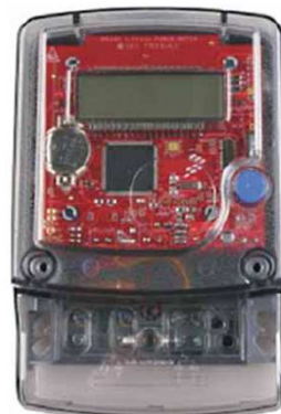
Secure pre-paid meter using MK30 MCU
