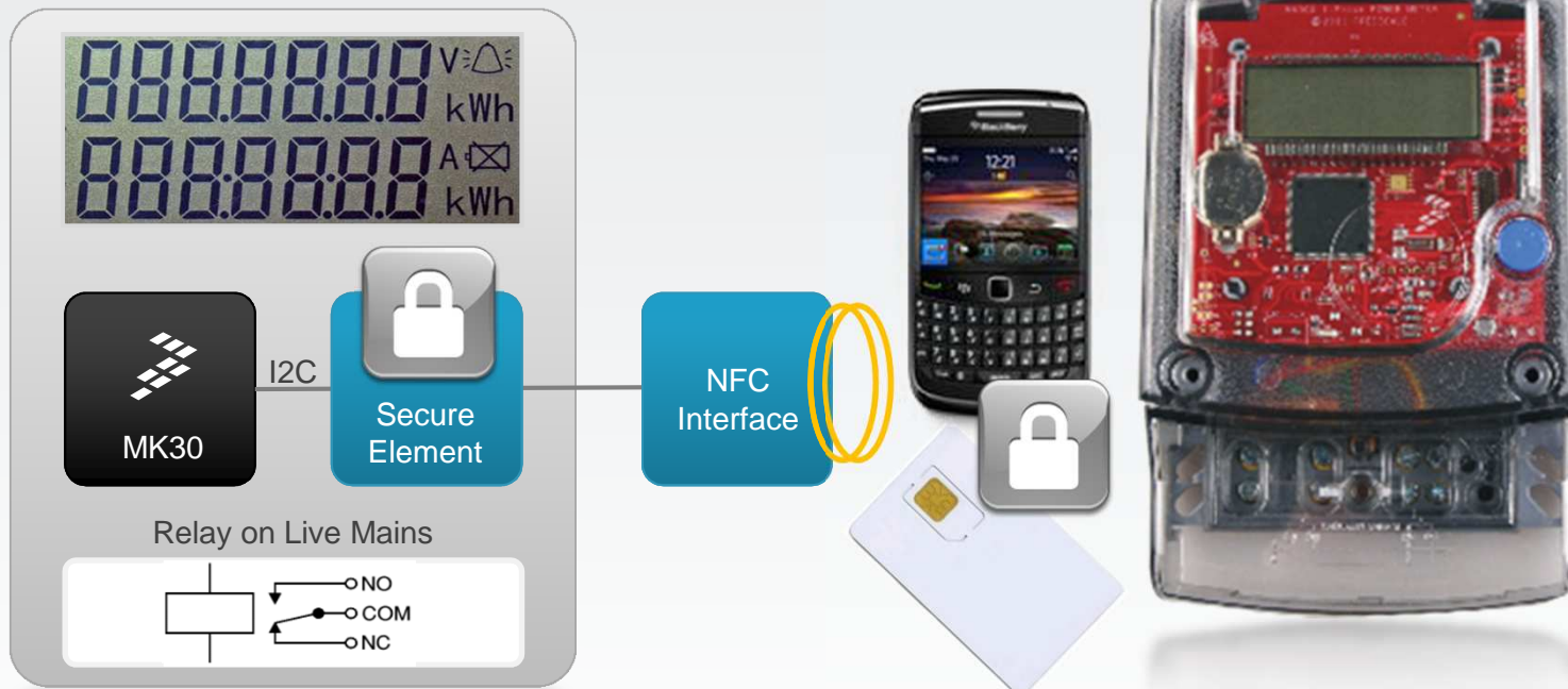
Basic components of a secure prepaid meter
