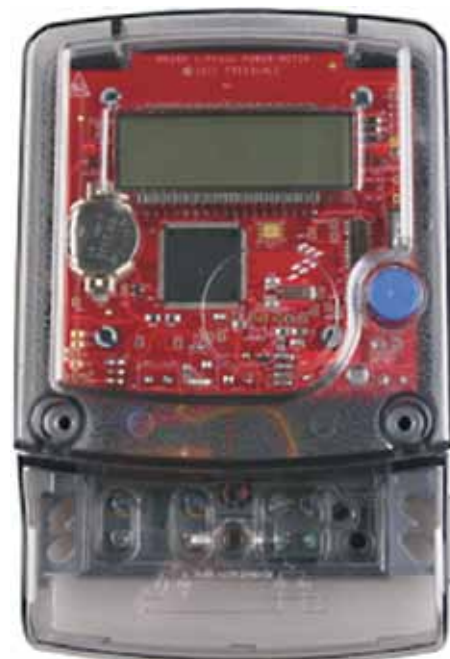
Secure prepaid meter using MK30 MCU
