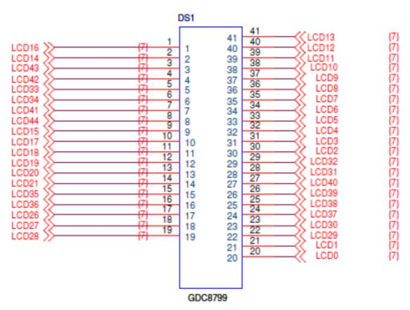
Figure 6. Segment LCD schematic
