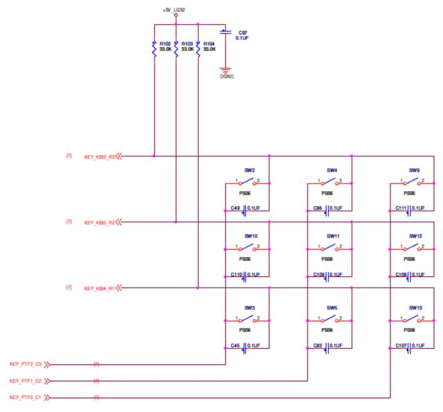
Figure 2. Matrix keypad schematic
