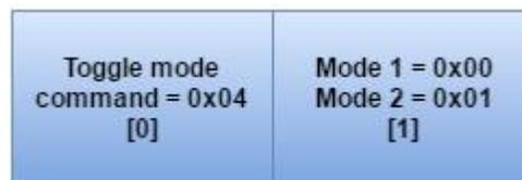
Figure 4. Toggle mode command frame
