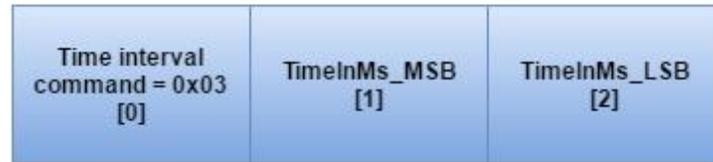
Figure 3. Change time interval command frame
