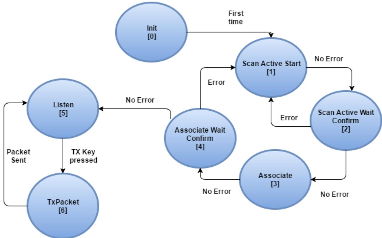
Figure 8. End device application state machine
